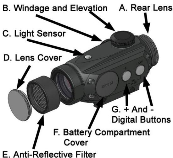
**A.** Rear Lens; **B.** Windage and Elevation; **C.** Light Sensor; **D.** Lens Cover; **E.** Anti-Reflective Filter; **F.** Battery Compartment Cover; **G.** + and - Digital Buttons;
