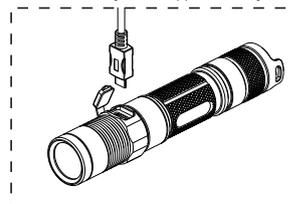
Under normal charging conditions, the blue power indicator light will illuminate steadily to notify users. When charging is complete, the MH12 will terminate the charging process automatically and the blue power indicator goes out.
